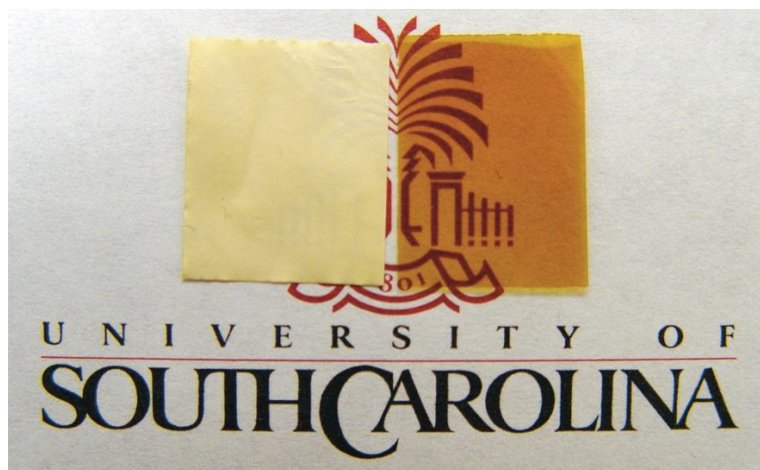
Figure 3.12 BTBP-PBI dense films ( left : dried under air; right : dried under nitrogen)
