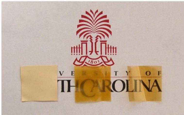
Figure 4.6 6F-PBI free-standing films prepared by various methods ( left : prepared with 3 wt% 6F-PBI/DMAc solution in open air; middle : prepared with 3 wt% 6F-PBI/LiCl/DMAc (PBI: LiCl=1:0.3, w:w) under dry nitrogen protection; right : prepared with 3 wt% 6F-PBI/DMAc solution under dry nitrogen protection).
